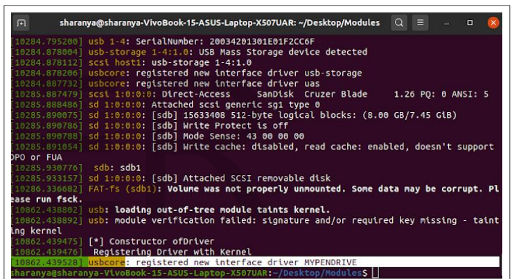
Fig 4: Pen-drive gets registered by the device driver
